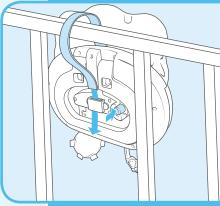
**TO RELEASE MIRROR Press release button** and pull strap up.
